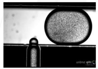
Fig. 6: Cell encapsulation process into a droplet
